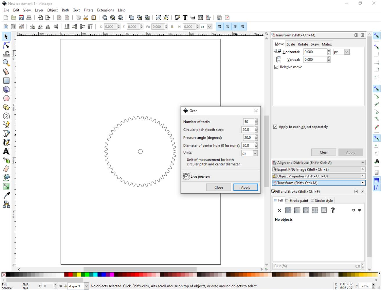
Using Inkscape to design a Spirograph. Step 2: The Gear window will pop-up where one can fill in various parameters of the gear to draw. The most important one is the Number of teeth. Once a large outer gear and two or more smaller gear outlines are drawn then one can make inside them small holes in various positions where the tip of the pen or pencil can go through
