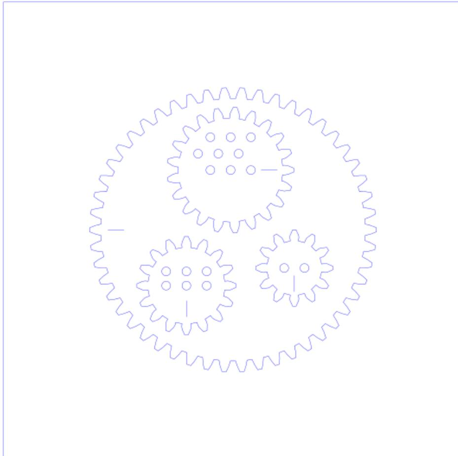
Spirograph with gears of 50, 21, 16 and 12 teeth than can be laser cut
