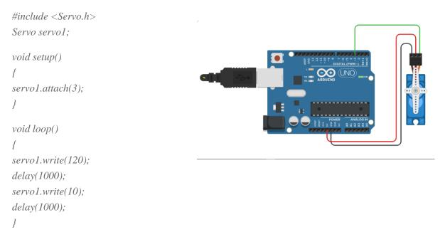
This code turns the servo to position 120 degrees, waits a second, turns it to position 10 degrees, waits a second and loops
