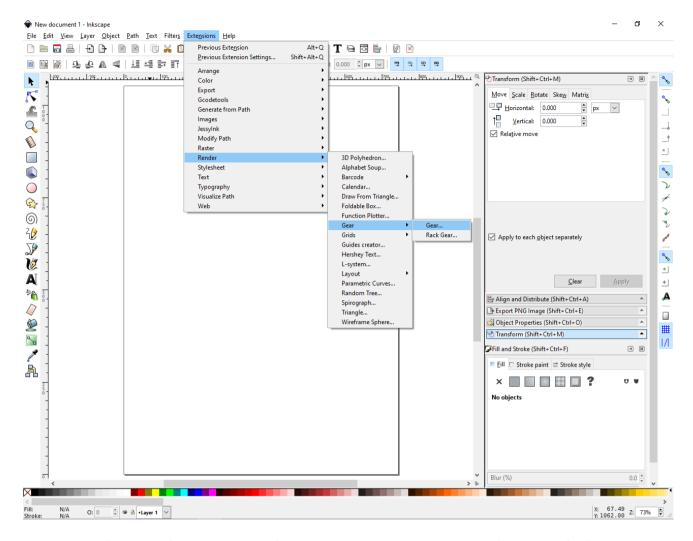
Using Inkscape to design a Spirograph. Step 1: First Go to Extensions/Render/Gear and select Gear
